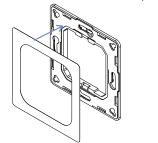
**Method 1**:Stick 3M glue on the back of the bracket and then stick the bracket to the wall
