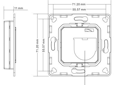
Battery: CR2450 | Before the first use, please open the battery cover and remove the protective film
